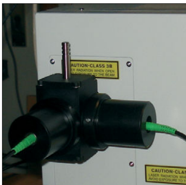
Fig. 1: Polarization extension mounted at the exit port of a Olympus Fluoview FV1000 scan head.
