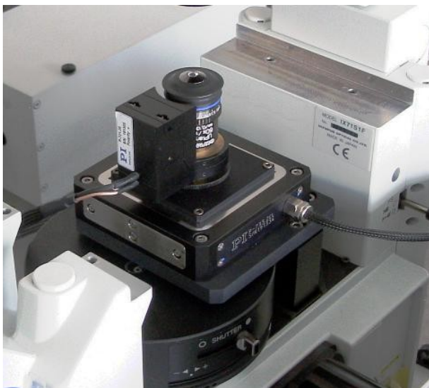
Fig. 1: The MicroTime 200 is used in objective scanning mode, in which the objective is mounted directly on the scanner and moved below the stationary sample.
