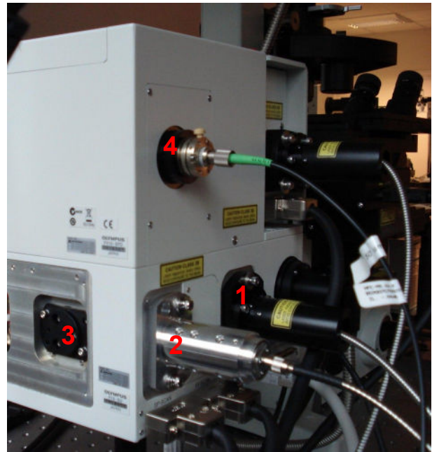
Fig. 4: Guiding CW and pulsed light into the FV1000 scan head: CW light delivery fiber with collimator (1), pulsed light delivery fiber with collimator (2), polarizing beamsplitter holder (3), fluorescence exit port with fiber coupling for external detector for FLIM, FCS, etc..(4)
