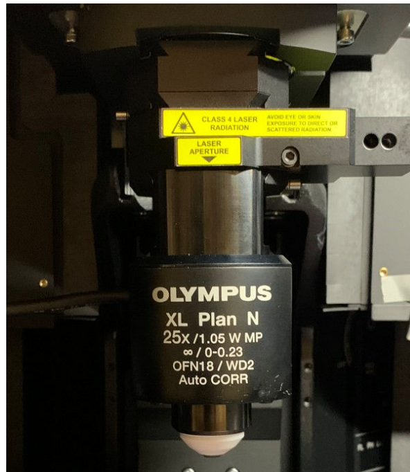
Fig. 2: Nosepiece adapter (with yellow laser warnings) for NDD FLIM measurements on upright microscopes
