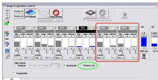
Fig. 3: Screen shot of the LSM software. The two red circled detectors can be used for NDD FLIM if the Photon Counting mode is activated in the Image Acquisition Control window (green circle).
