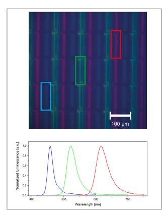
Figure 7: Top: microscopy image of a smartphone screen captured through a 20x objective. The blue, green and red pixels selected for the measurements are indicated by boxes in the corresponding colors.
