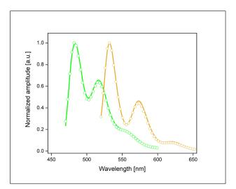
Figure 3: TRES recorded from the fluorescence polymer blocks SFG ( $\tau_n$  = 3.8 ns) and SFO ( $\tau_n$  = 3.5 ns)
