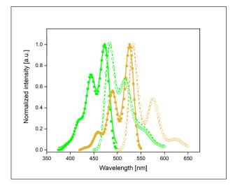
Figure 2: Excitation and emission spectra of the fluorescence polymer reference block SFG (green) and SFO (orange). Spectra obtained using the FluoMic add-on are shown as lines (solid = excitation, dashed = emission) and those recorded using a conventional sample holder as circles (filled = excitation, empty = emission).
