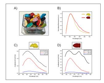
Figure 4: Gummy bears (A) and their spectral properties: steadysate spectra of a yellow and red gummy bear recorded upon excitation at 440 nm (B), TRES of the yellow gummy bear (C) and of the red one (D)
