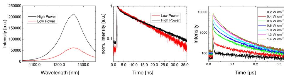
It is obvious that both PL spectra and decays are different depending on the excitation power. At higher excitation power the TRPL image of the sample is getting more homogeneous due to saturation of trap states inside the sample. The PL lifetime is significantly affected by the applied power density (see right graph). For carrier diffusion studies, a confocal setup is required. To avoid carrier dynamics, a widefield microscope with higher excitation densities is recommended.
