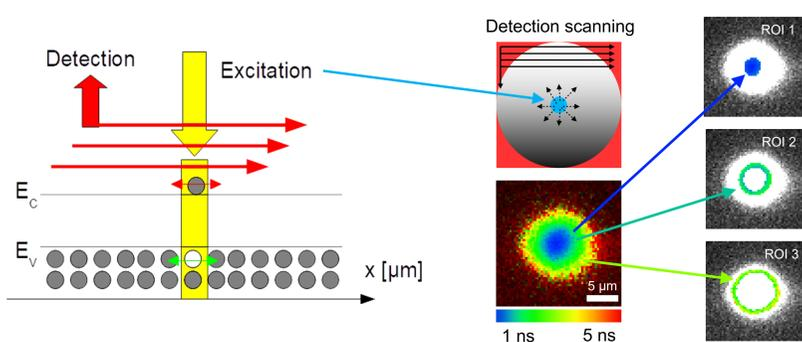
The time-resolved PL detection in combination with XY raster scanning of the **confocal detection** volume over the fixed excitation spot allows a direct observation of the carrier diffusion away from the fixed excitation spot in semiconductors.
