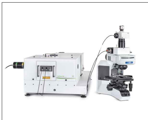
Figure 1: The FluoMic Microscope consists of a specialized sample mounting unit (A), a series of pre-aligned optical fibers (B), a fiber in-coupler (C) and out-coupler (D) unit that can be attached to various microscopes (here an Olympus BX43 is shown).
