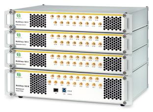
The MultiHarp 160 is designed as a plug-and-play event timer and Time-Correlated Single Photon Counting (TCSPC) unit which is optimized for applications that require a large number of fast and precise timing channels. The high quality and reliability of the MultiHarp 160 is reflected by our unique 5-year limited warranty.
