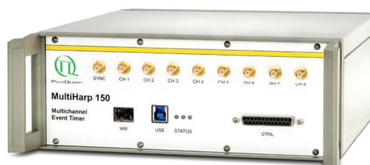
The MultiHarp 150 is an easy-to-use, plug-and-play multi-channel event timer and Time-Correlated Single Photon Counting (TCSPC) device. Its outstanding features are an extremely fast signal processing along with an extraordinarily high sustained data throughput via USB 3.0 interface. The MultiHarp 150 is a compact, robust and reliable device whose high quality is reflected by our unique 5-year limited warranty.
