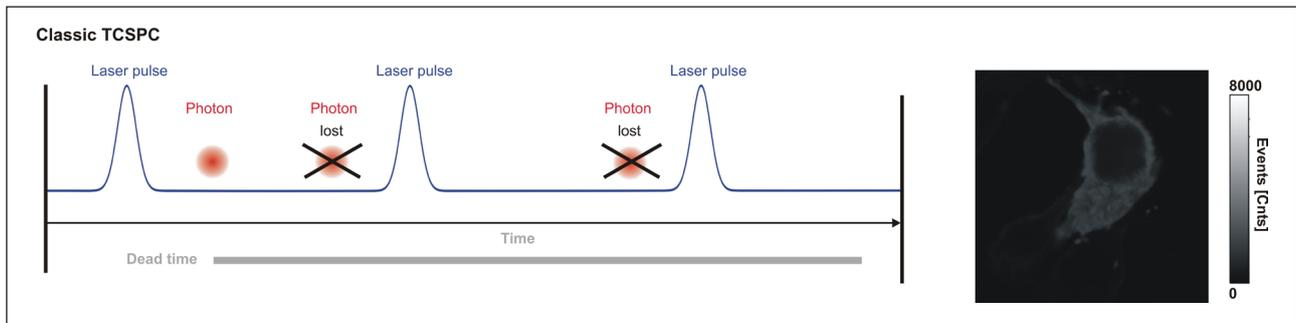
Figure 3A: Dead times in classic TCSPC electronics. Left: scheme of the interaction of laser pulses, dead times and detected photons. Right: FLIM intensity images of a cell recorded under classic TCSPC conditions.
