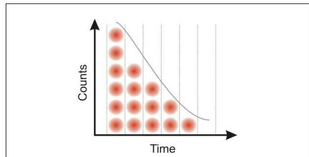
Figure 2: Histogram of start-stop times obtained from a TCSPC measurement. The discrete time bins (channels) are indicated by dashed lines.
