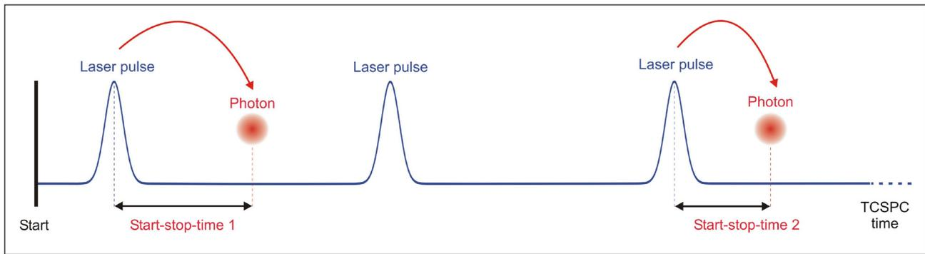
Figure 1: Recording photon arrival times in a time-resolved fluorescence measurement with TCSPC.
