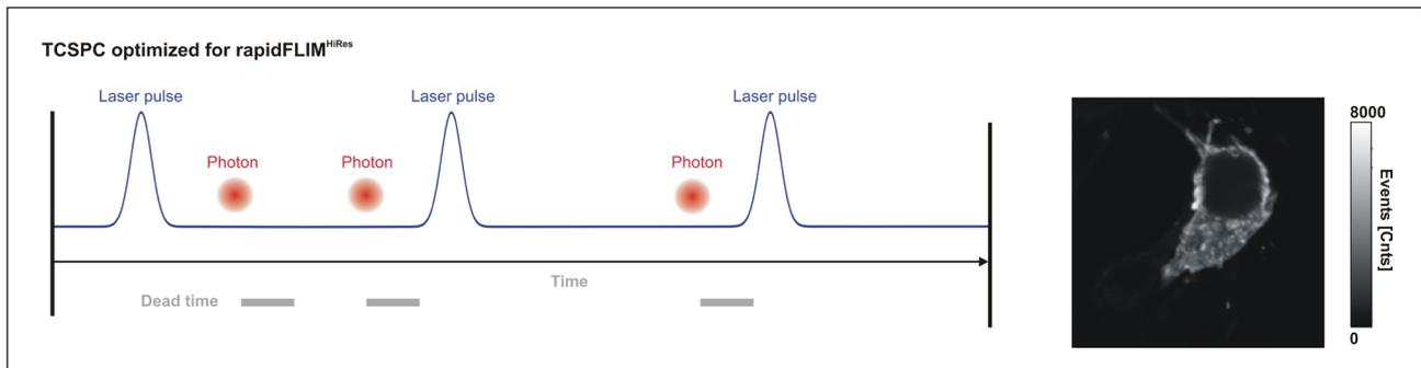
Figure 3B: Dead times in rapidFLIM<sup>HiRes</sup> optimized TCSPC electronics. Left: scheme of the interaction of laser pulses, dead times and detected photons. Right: FLIM intensity images of a cell recorded under rapidFLIM<sup>HiRes</sup> conditions.
