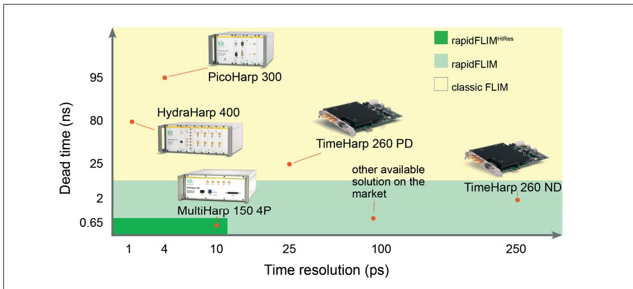
Figure 4: Dead times (y axis) and timing resolution (x axis) of PicoQuant's various TCSPC electronics and comparison with other commercially available solutions.
