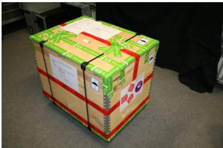
Fig. 48: Adding warning labels, schockwatches, and sealing with adhesive tape
