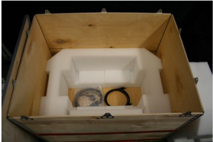
Fig. 40: Orientation of the bottom foam brackets in the box
