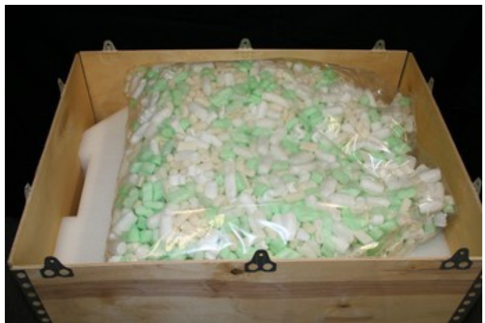
Fig. 44: Filling up the empty space with styrofoam chips
