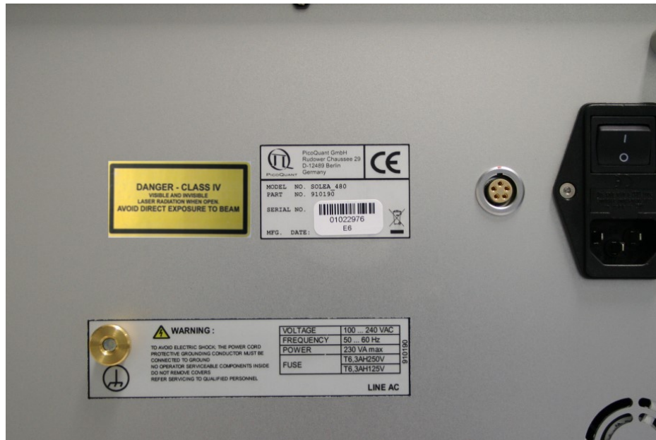
Fig. 2: Warning and classification label, as well as identification label on the back panel.
