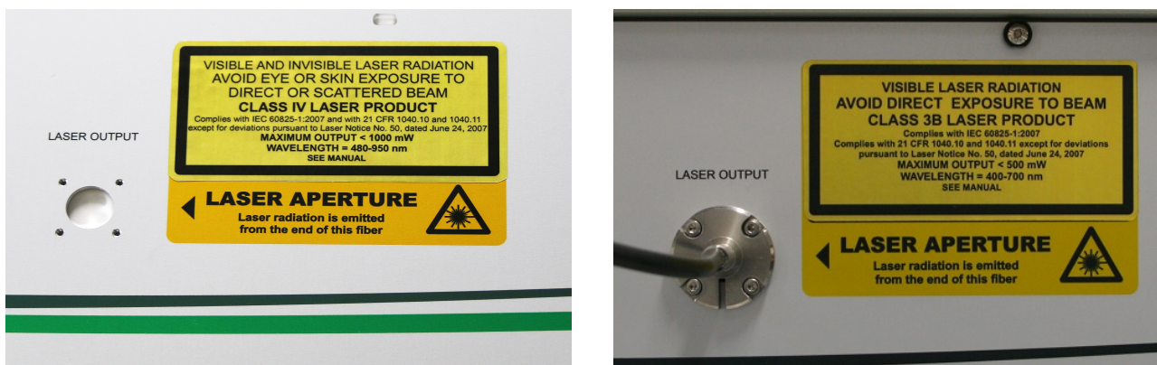
Fig. 1: Laser aperture, laser warning, certification and laser classification label. Left: for class 4 / IV laser product (SoleaR and Solea White); Right: for class 3B / IIIB laser products (Solea and Solea White).
