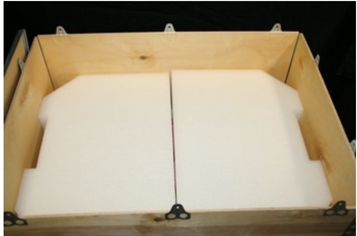
Fig. 43: Placing the top foam brackets
