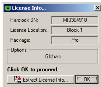
The serial number of the Hardlock module, the location of the current license and the software package available are shown in the upper region of the dialog. Currently there are two packages available for FluoFit, called "Basic" and "Pro".
