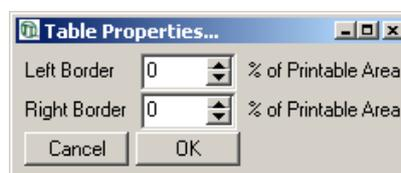
The width and height are entered in percent of the printable region, which is the width of the report page minus the margins. Likewise, the table border distances are measured from the margins, i.e. "0% left and right border" means that the table will be exactly as wide as the printable area.
