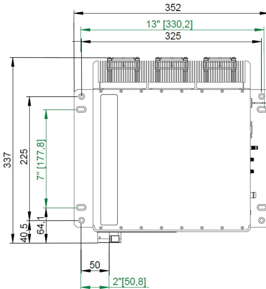
**Dimensions of the VisIR-AC laser module with shutter:**
