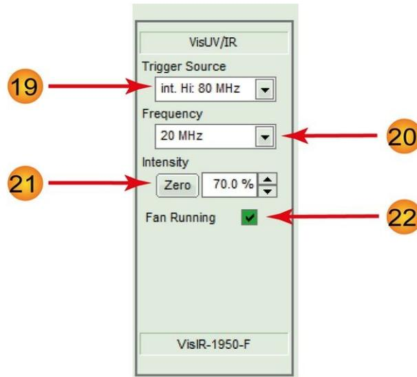
Fig. 21: VisUV/IR laser control elements in the GUI
