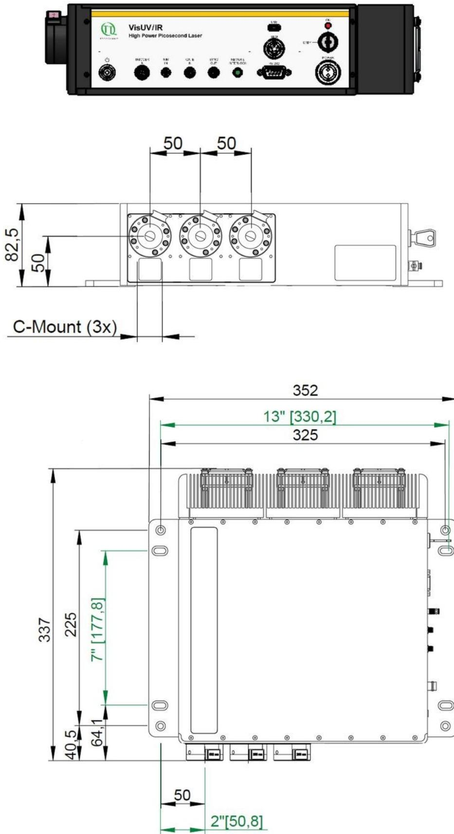
**Dimensions of the VisIR/VisUV laser module with filter holder:**
