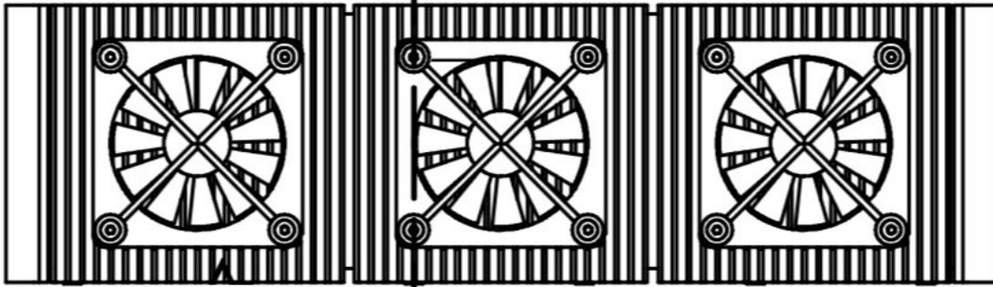
Fig. 12: Heat sink with integrated fan aperture
