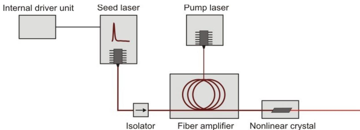
Fig. 5: VisIR – Schematic representation of the working principle
