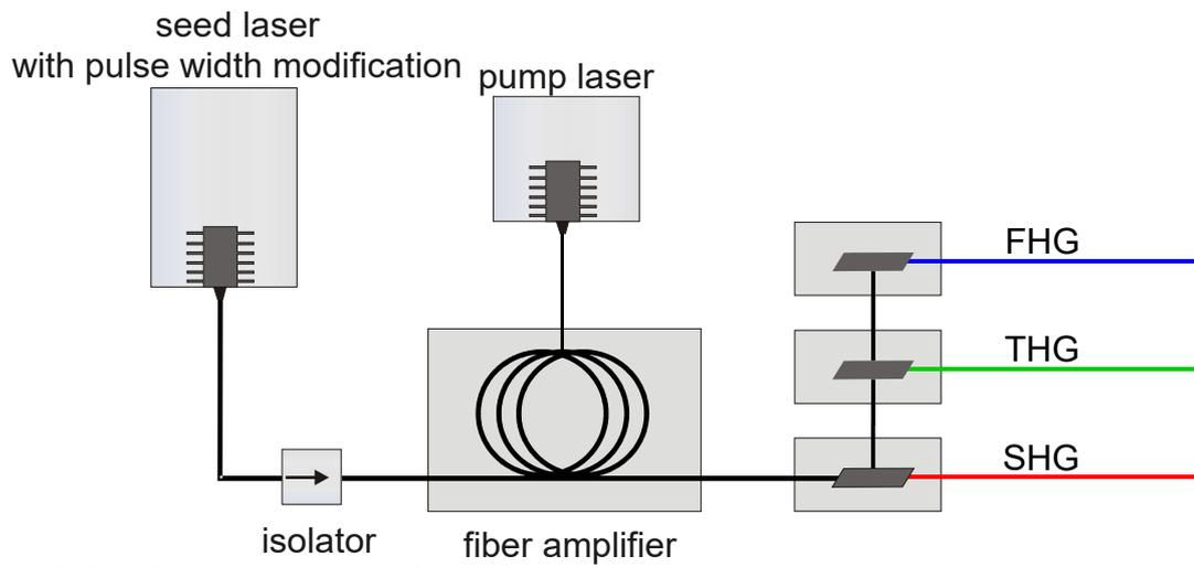
Fig. 6: VisUV - schematic representation of the working principle
