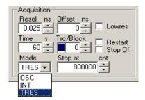
A TRES measurement is started or canceled as usual via the toolbar buttons for start and stop. The data acquisition will be performed like a standard "Integration Mode" measurement, while the block number is incremented for each new wavelength.
