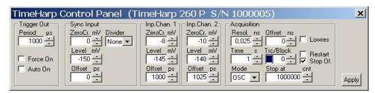
The control panel sections and their respective controls are listed below, indicating differences of the two hardware versions (PICO/NANO) where they apply.
