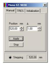
If there is a large difference between the current monochromator position and the position entered, the movement will take some time. If you wish to interrupt this process, press the *Stop* button. The monochromator immediately will slow down and stop. The deceleration is necessary to preserve the calibration.
