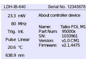
By accessing this menu option, the Taiko PDL M1 will display various information on the driver and connected laser head. Namely: the device type, part and serial numbers, the control module type CM as well as hardware and firmware versions.
