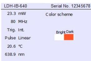
The toggle switch on this screen allows changing from the (default) bright to the dark color scheme for the local interface. The switch is operated by turning the dial.
