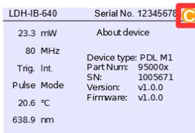
A calibration expired icon (orange circle with white “C” letter) will be shown in the upper right corner of the display once a laser head has exceeded a threshold in operating hours (laser diode dependent). Beyond this threshold, the calibrated power values can no longer be guaranteed. The deviation between the true value of emitted optical power and the displayed mW value might now lie above +/-10%.
