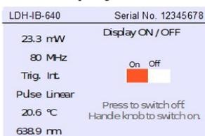
This setting screen allows turning the local LCD display on or off. Select the desired option and press on the dial to confirm your choice. The display can be reactivated by pressing the dial when the Taiko PDL M1 is on.
