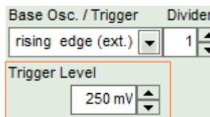
Fig. 46: Setting trigger level
