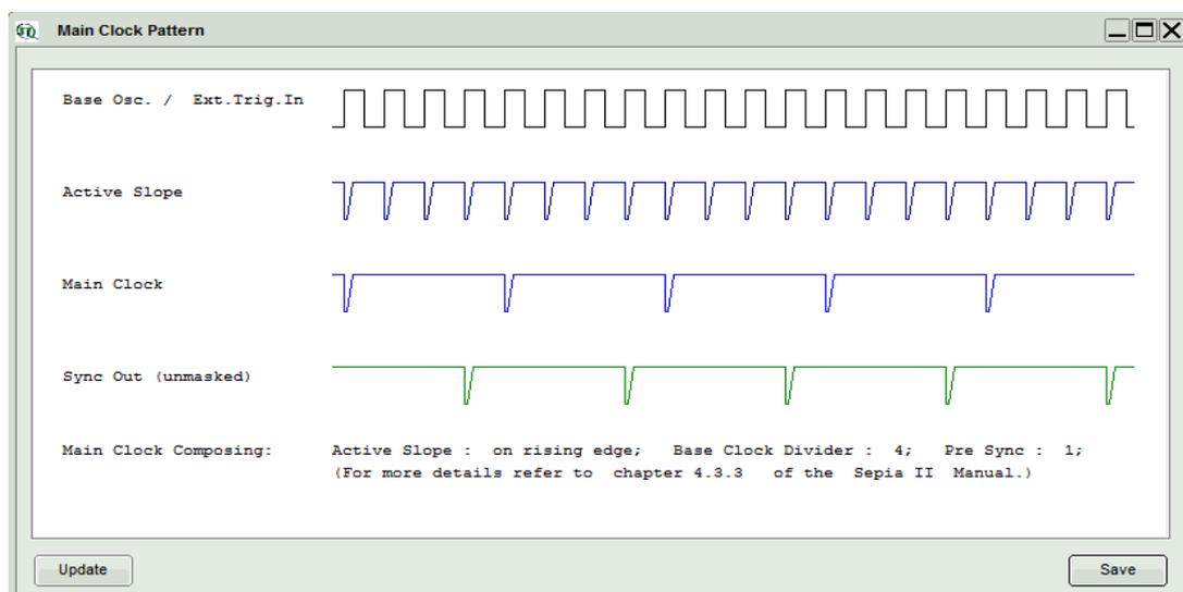
Fig. 47: Visualization of the Main Clock as set in Fig. 44
