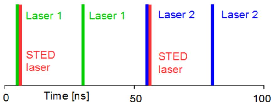
Fig. 63: PIE-STED pulse sequence involving two excitation lasers (blue and green) and a STED depletion laser (red).
