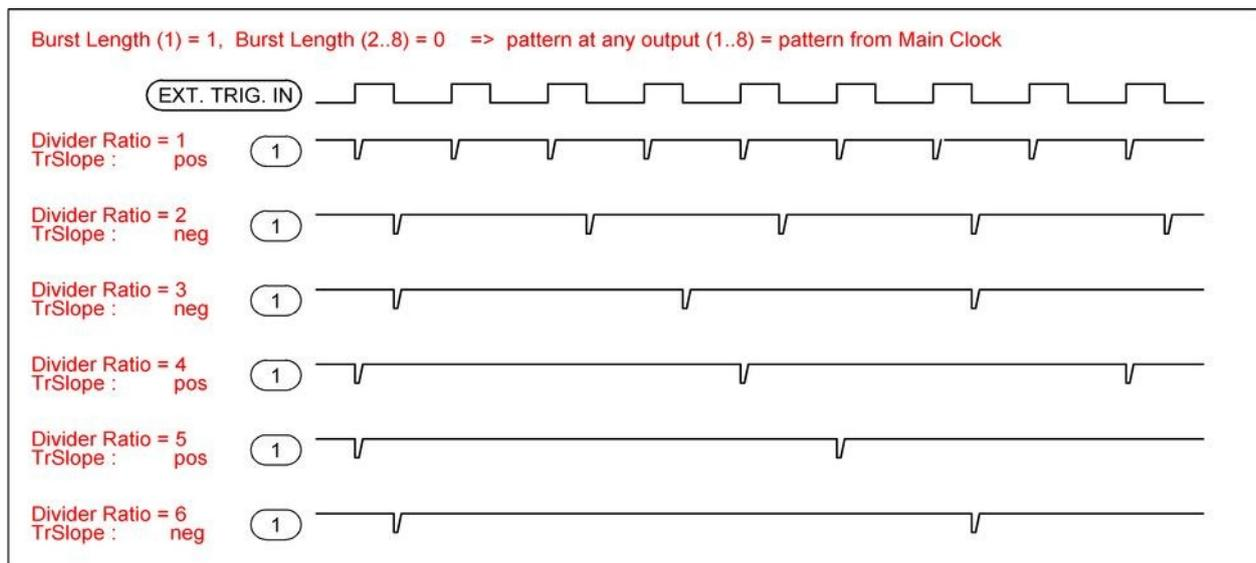
Fig. 25: Pattern from main clock at various divider settings
