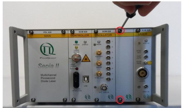
Fig. 33: Loosen the screw holding the metal plate.
