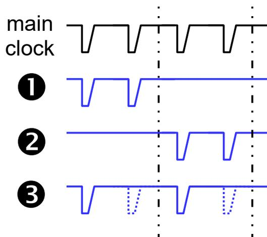
Fig. 65: Effect of activating 1st only for the STED burst channel (masked pulses are shown as dotted lines)
