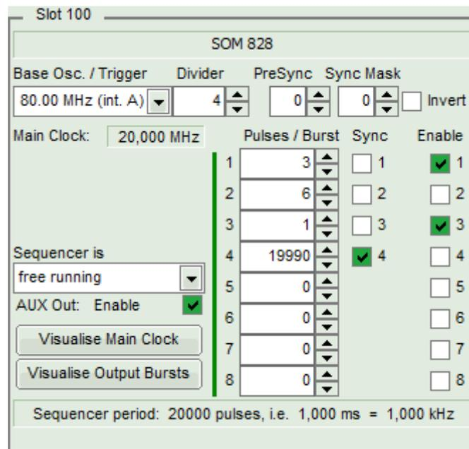
Fig. 58: Setting the SOM 828 to generate the example configuration
