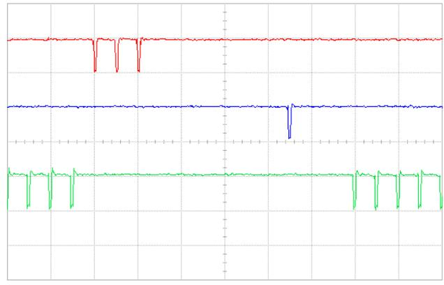
Fig. 60: Sync Mask = 2: leading two sync pulses are suppressed
