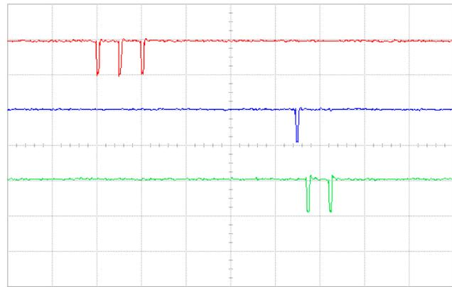
Fig. 62: Pre Sync = 2: Sync pulses are left-shifted against burst pulses
