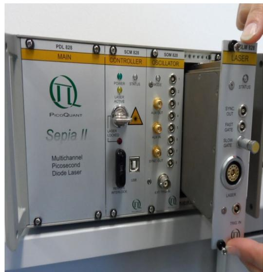
Fig. 36: Inserting the new module into the PDL 828 mainframe
