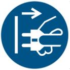
Disconnect the power cord from the electrical outlet before performing any maintenance.
