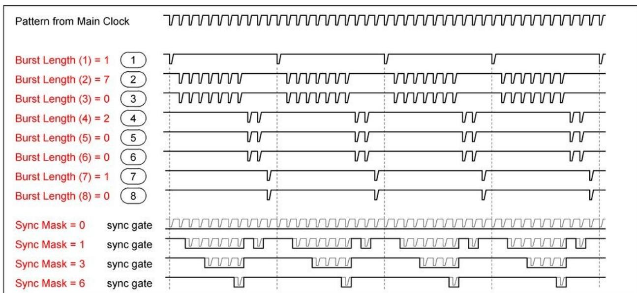
Fig. 26: Gating of synchronization pulses is controlled by the sync mask parameter
