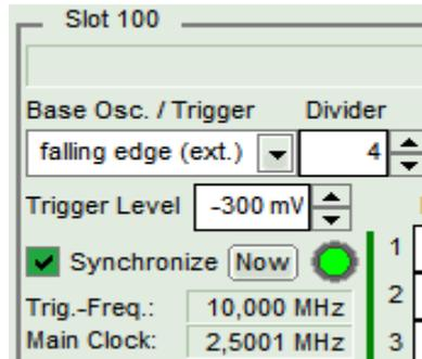
Fig. 51: Extended settings for external triggering - SOM 828-D
