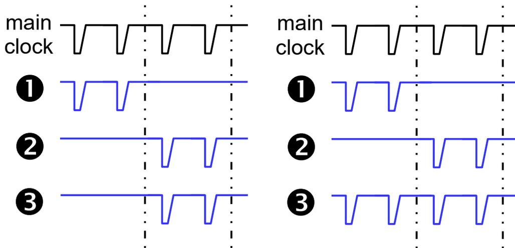
Fig. 64: PIE-STED pulse pattern after definition of burst channels and lengths (left part) and combination (right part).
