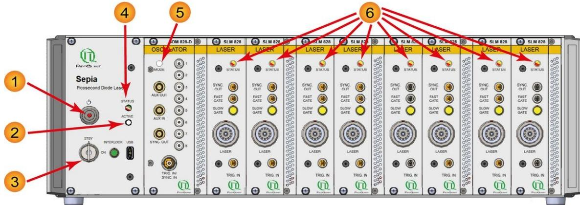
Fig. 19: Sepia PDL 828 Type "L" with SOM 828 module and eight SLM 828 modules
