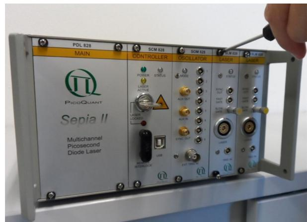
Fig. 37: Fix the screws of new laser driver module
