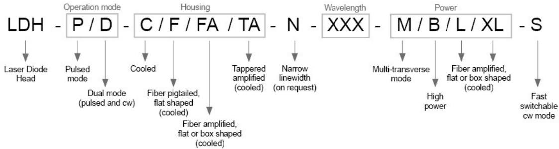
Fig. 67: PicoQuant laser head naming convention
