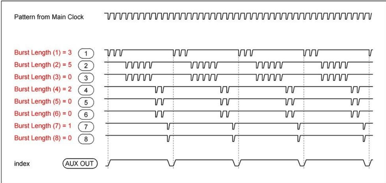
Fig. 28: Index pulse at start of the sequencer period
