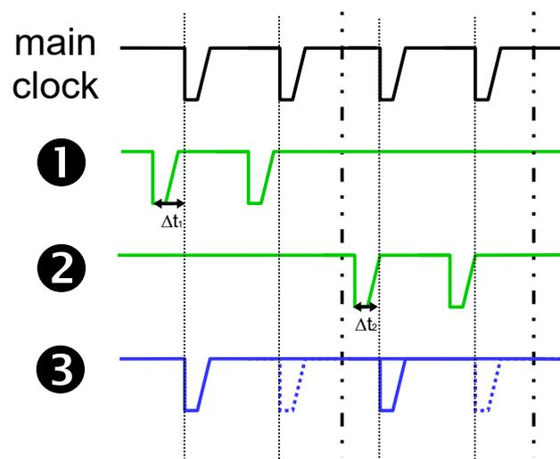
Fig. 66: PIE-STED pulse pattern with delays between excitation and STED laser pulses ( $\Delta t_1$  and  $\Delta t_2$ ). The thin dotted lines indicate the time points corresponding to the main clock pulses. The dash-dotted lines group pulses to individual bursts.
