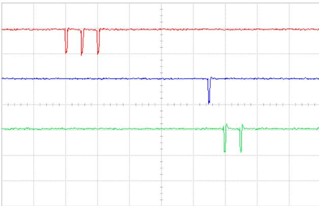
Fig. 61: Sync Mask inverted: leading two sync pulses are enabled
