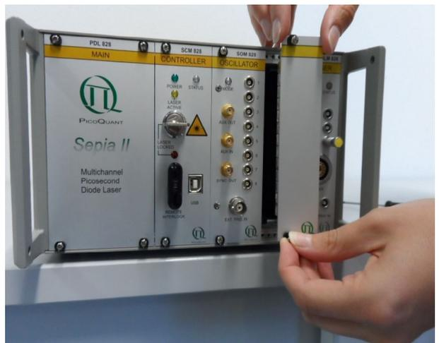
Fig. 34: Carefully remove the metal plate.
