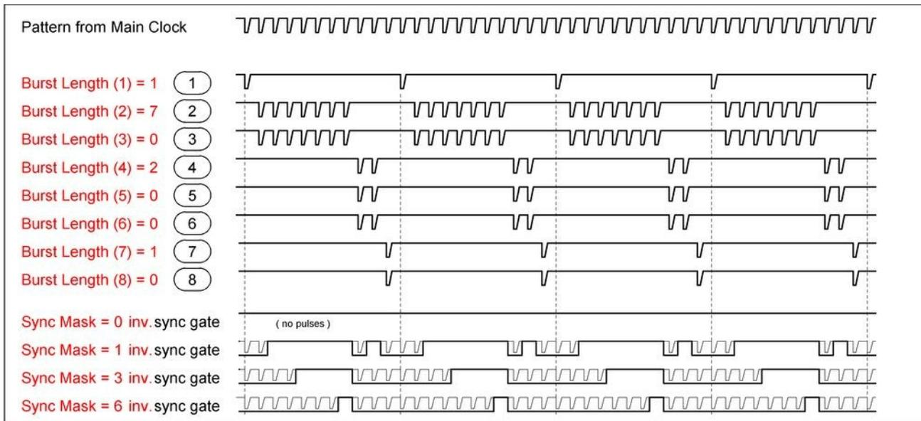
Fig. 27: Synchronization patterns resulting from an inverted sync mask
