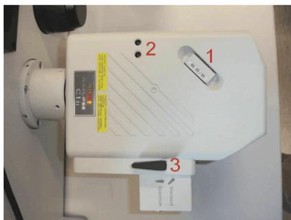
**Fig. 2.1:** The Nikon C1si/C2 scan head. 1: dichroic, 2: pinhole adjustment, 3: switch for “standard” and “spectrum” detection. FLIM and FCS is performed with the “spectrum” setting.
