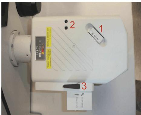
**Fig. 2.9:** The Nikon C1si/C2 scan head. 1: dichroic, 2: pinhole adjustment, 3: switch for “standard” and “spectrum” detection. FLIM and FCS is performed with the “spectrum” setting.
