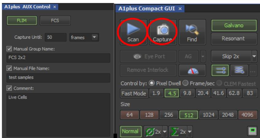
**Fig. 2.5:** Selection of a FLIM measurement up to 50 frames, and controls to start the measurement. “Scan” makes a test measurement, which is not saved, and “Capture” makes a final measurement which is saved.
