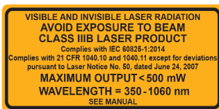
Fig. 1.4 Class IIIB Laser Power and Wavelength Specifications Label on the side of the LCU (B)
