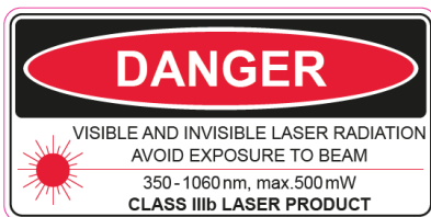
Fig. 1.5 Class IIIB Laser Power and Wavelength Specifications Label (US) on the side of the LCU (D)
