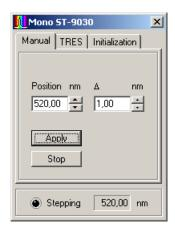
If there is a large difference between the current monochromator position and the position entered, the movement will take some time. If you wish to interrupt this process, press the *Stop* button. The monochromator immediately will slow down and stop. The deceleration is necessary to preserve the calibration.
