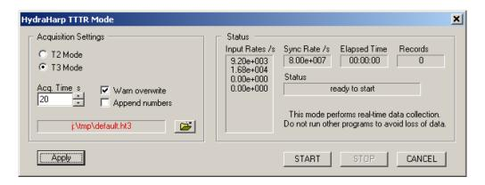
The dialog section *Acquisition Settings* is for the selection of the measurement mode (T2 / T3), an overall acquisition time and a file name. Note that switching between T2 and T3 mode takes some time because the hardware must be reconfigured. Normally such a switching should not occur often because the two modes usually require a very different experiment setup.
