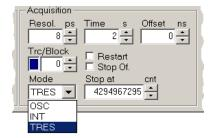
A TRES measurement is started or canceled as usual via the toolbar buttons for start and stop. The data acquisition will be performed like a standard "Integration Mode" measurement, while the block number is incremented for each new wavelength.
