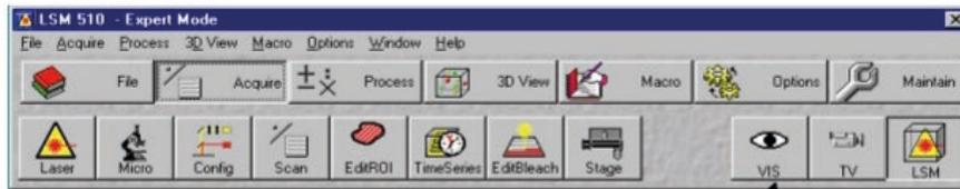
To view the sample through the eyepiece, click on "VIS". Toggle between VIS and LSM button in main menu to automatically switch between direct observation and laser scanning
