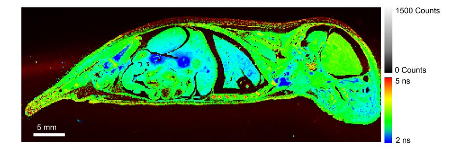
Sample: unstained mouse embryo Data acquired with: MicroTime 100, equipped with a widerange scanner  $I_{exc} = 485 \text{ nm}, 20 \text{ MHz}$  $I_{det} = 530 \text{ nm} - 550 \text{ nm}$ Hybrid-PMA detector Pixel time: 5 ms Aquisition time: 22 min 800x300 pixel, 2x2 binning
