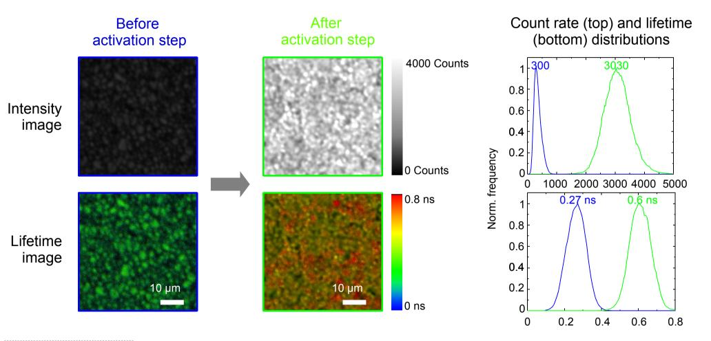
$λ_{exc}$  = 635 nm, 40 MHz  $λ_{det}$  = 814 - 870 nm τ-SPAD detector
