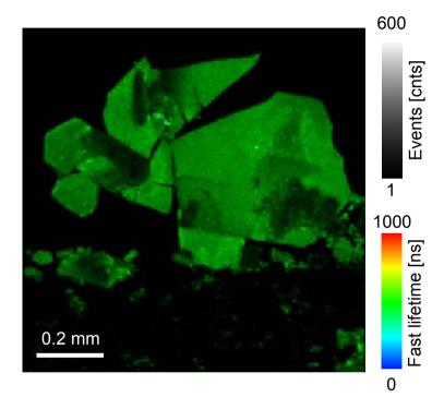
Sample: RuBiPy (Tris(bipyridine) ruthenium(II) chloride) crystals Data acquired with: MicroTime 100  $\lambda_{\text{Exc}}$ : 375 nm, 0.5 MHz UPlanSApo 10x, NA 0.4 Time/pixel: 0.9 ms Image size: 1 x 1 mm (200 x 200 pixel) Total recording time: 120 s Emission filter: HQ500LP Detector: Hybrid PMT
