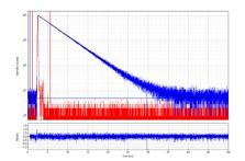
Fluorescence lifetime measurements of ATTO 555 in ethanol. The sample was excited at 550 nm using a spectral bandwidth of 5 nm and a repetition rate of 20 MHz. Data was collected using the TCSPC based spectrometer FluoTime 300. Data analysis using numerical reconvolution resulted in a single liftetime of 3.87 ns (c2=1.07).
