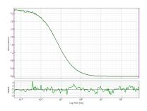
Fluorescence correlation spectroscopy (FCS) of ATTO 655 in water. The sample was excited at 630 nm using a spectral bandwidth of 5 nm and a repetition rate of 10 MHz. Data was collected using the confocal microscope MicroTime 200. The correlation curve can be nicely fitted and the amplitude of zero at long lag times proves the high stability of the laser output.
