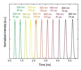
Pulse profiles and pulse widths (FWHM) at different central wavelengths after the emission wavelength selector. The spectral bandpass was set to 5 nm.
