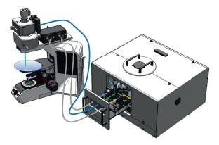
In many cases, characterizing materials such as semiconductors or solar cells requires measuring their photophysical properties at various points with spatial resolution. However, scanning over a large sample area is often not needed, as point measurements at various sites are sufficient.
