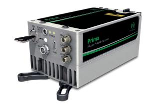
Prima is a compact, stand-alone and affordable laser module offering 3 individual emission wavelengths that can be operated in picosecond pulsed and continuous wave (cw) mode. The picosecond pulses can be triggered either by the module's internal clock or by an external oscillator at up to 200 MHz. The module is fully computer controlled, making its operation very easy: Connect Prima to a PC via an USB port and all changes in operation parameters can be done via a convenient software interface.
