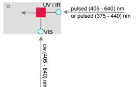
Fig. 2: Coupling of pulsed lasers into the FV300 scan head. The polarising beam splitter is shown in red. The UV / IR port accepts either the wavelengths range (405 – 640) nm or (375 - 440) nm, because different collimators have to be utilized for the two wavelengths ranges. If the UV / IR port is blocked by a different laser, please as PicoQuant for advice.
