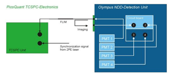
Fig. 2: Schematic overview of a four-channel NDD FLIM set-up. In this scheme, the cabling modification just for PMT 1 is shown.
