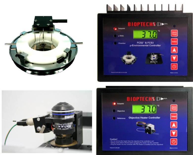
Fig. 1: Assembled Microfluidic flow cell (FCS2, above) and microscope objective heater (below) along with their corresponding controllers
