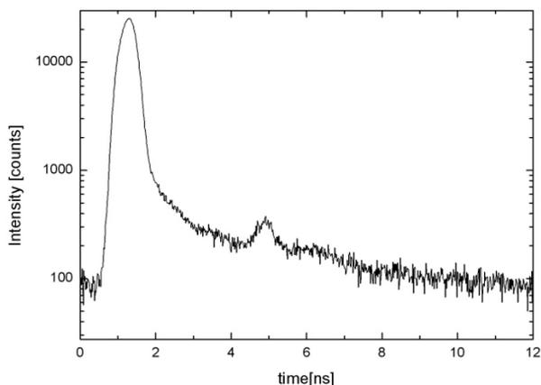
Fig. 4: Measurement of the instrument response function (IRF) via SHG in collagen samples using the internal NDD PMTs operated in photon counting mode. An IRF of 500 ps was obtained with a clearly visible reflection approx. 3 ns after the main peak. The decaying tail of the IRF is due to residual fluorescence from the collagen sample.
