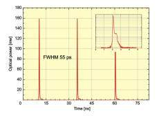
The PDL 800-B is a stand-alone driver for the picosecond pulsed laser diode heads from 375 to 1990 nm (LDH-P/FA Series) as well as for the sub-nanosecond pulsed LEDs from 255 to 600 nm (PLS Series). The laser heads can emit light pulses as short as 70 ps FWHM (50 ps on selection) at repetition rates from single shot up to
