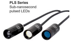
Available wavelengths: 255-600 nm, options: spectral bandpass filter
